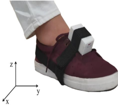
Figure 2. Foot-mounted IMU placement used in the GSTRIDE dataset [27].
