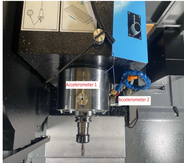
Figure 5. The piezoelectric accelerometers attached to a Hurco VMX42Di CNC machine.
