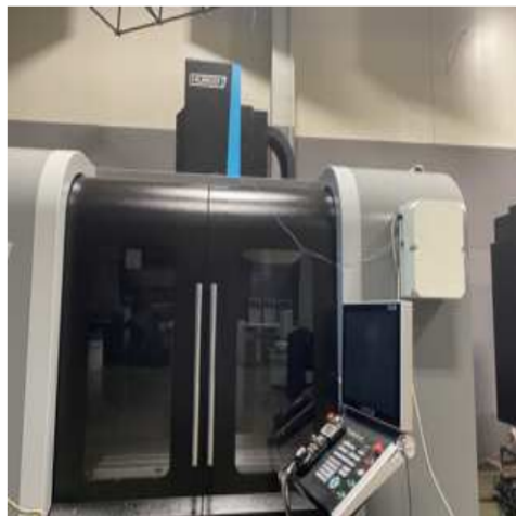
Figure 4. The plastic control box mounted onto a Hurco VMX42Di CNC machine.
