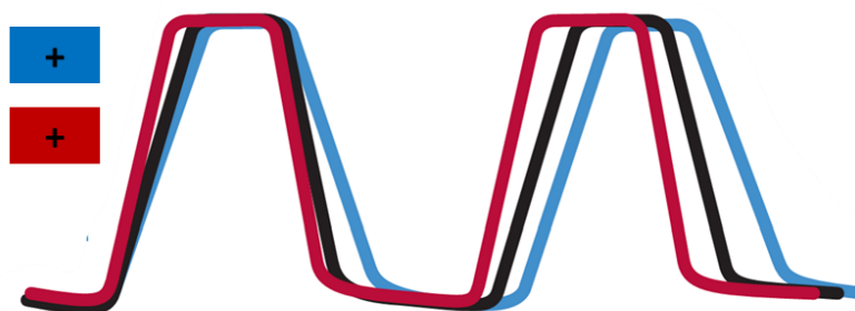
Figure 4. Effect of UltimArc™ parameter on frequency waveform in P-GMAW process.
