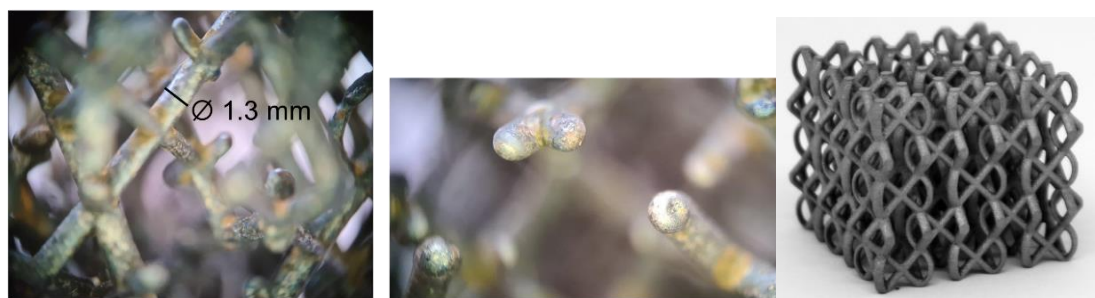
Figure 7. Left, middle: cold runs; right: sample with sandblasted surface in scale 1, variation 1.
