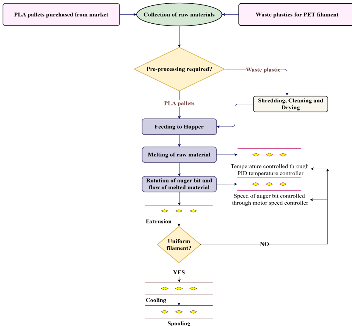
Figure 2. Overview of filament extrusion process.
