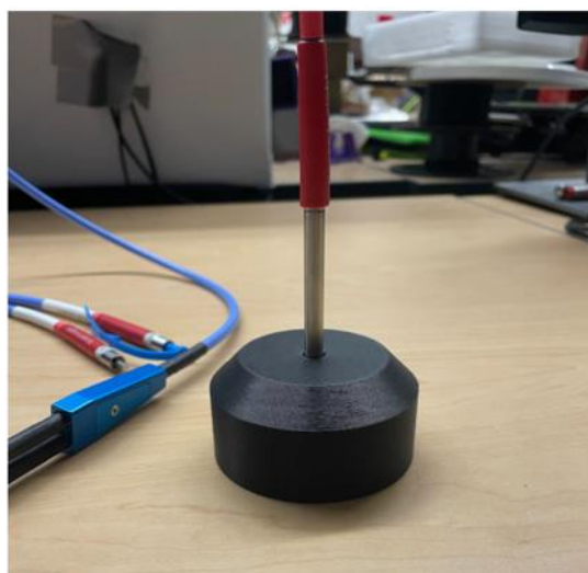
Figure 4. 3-D printed probe holder.
