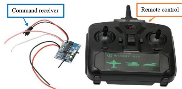
Figure 5. The remote control of the robotic system prototype for water analysis.
