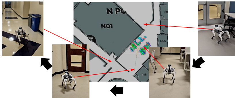
Figure 10. The robot localizes directly on the floor plan image and performs a navigation task. The occupancy grid map that the robot used for localization and navigation was also derived from the floor plan map captured by the robot. We manually removed the labels that would otherwise be interpreted by the robot as obstacles. From right to left, the robot was performing (1) Going through Door N09, (2) Approaching Door N00, (3) Opening Door N00, and (4) Approaching Door T01.
