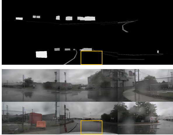
Figure 13. Generating result of a rainy day after removing the center line in the rear camera.
