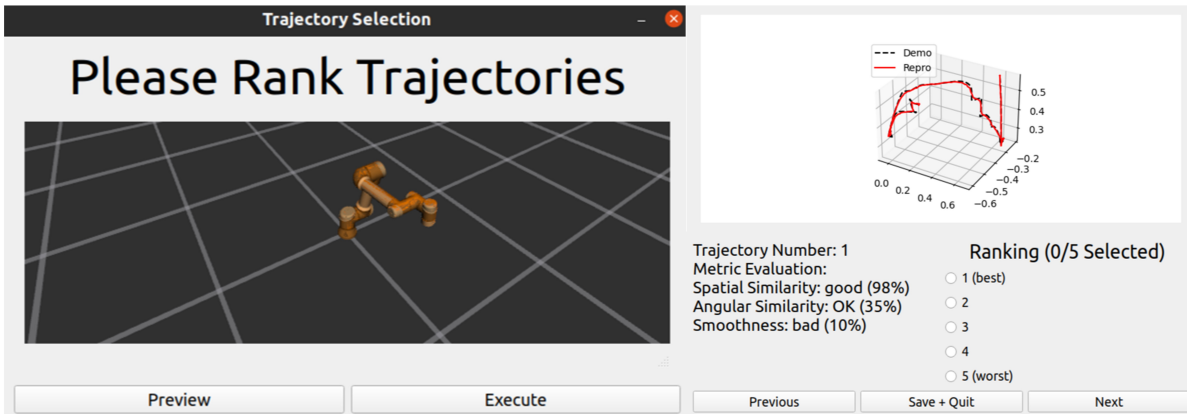
Figure 7. The GUI used to allow users to rank their preferred reproductions. Users were asked to rank five reproductions, three of which minimized each objective in Equation (8), one which mixes these objectives similar to user preferences, and one sub-optimal reproduction which does not lie on the Pareto front.
