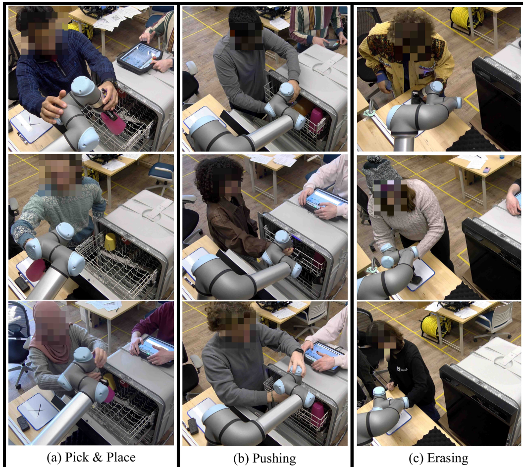
Figure 8. The three tasks used in our user study: (a) pick & place; (b) pushing; and (c) erasing letter “S”.
