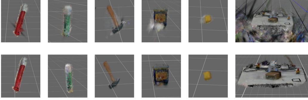
Figure 3. Qualitative results of the point cloud cleaning pipeline. Top: Raw 3DGS point clouds exhibit floaters and surface fuzziness, which impede precise collision checking. Bottom: Refined geometries after applying our multi-stage filtering, including heuristic filtering and DBSCAN. The process effectively removes artefacts and sharpens boundaries, yielding planning-ready digital twins for manipulation tasks.
