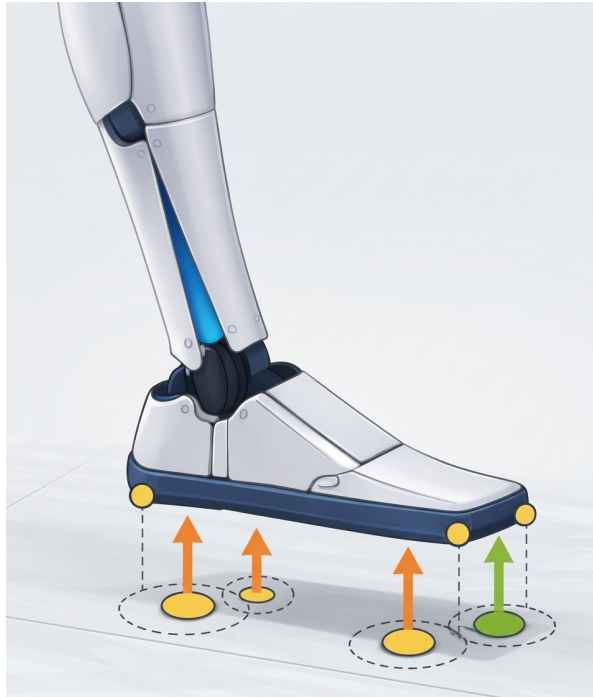
Figure 1. Foot corner contact modeling diagram.
