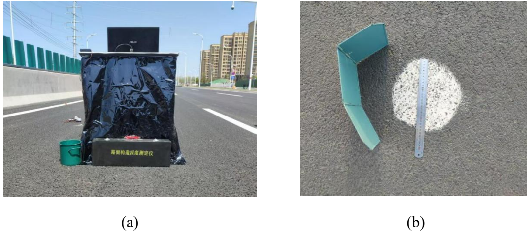
Figure 3. Process of data collection. (a) Mobile setup for image recording; (b) Texture depth measurement.
