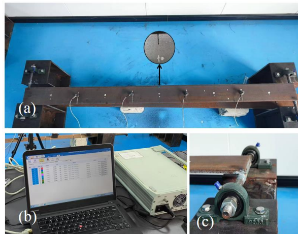
Figure 10. Experimental setup. (a) Simply supported beam and damage location; (b) Data acquisition system; (c) Ball bearing support.
