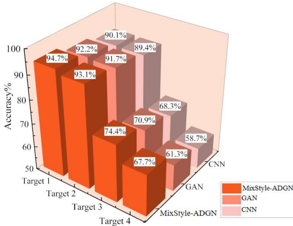
Figure 5. Damage-localization accuracy of the CNN, domain-adversarial baseline, and MixStyle-ADGN models in the four target domains.
