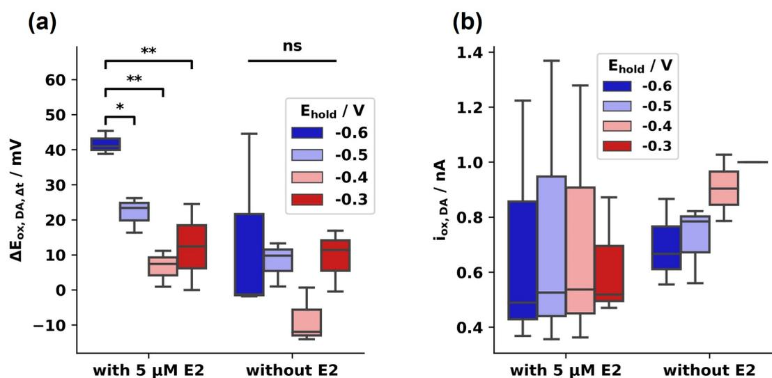
**Figure 11.** DA detection kinetics when detected with *vs.* without E2. **(a)** From 7 s to 15 s, a shift of  $E_{ox,DA}$  to higher potentials occurs both when DA is detected with E2 and without the presence of E2. However, the shift increases significantly when  $E_{hold}$  is decreased when DA is codetected with E2. **(b)**  $i_{ox,DA,7s}$ . Post-hoc Tukey 95%, \*:  $p < 0.05$ , \*\*:  $p < 0.01$ , \*\*\*:  $p < 0.001$ .  $n = 5$  in codetection  $n = 3$  in DA detection alone.
