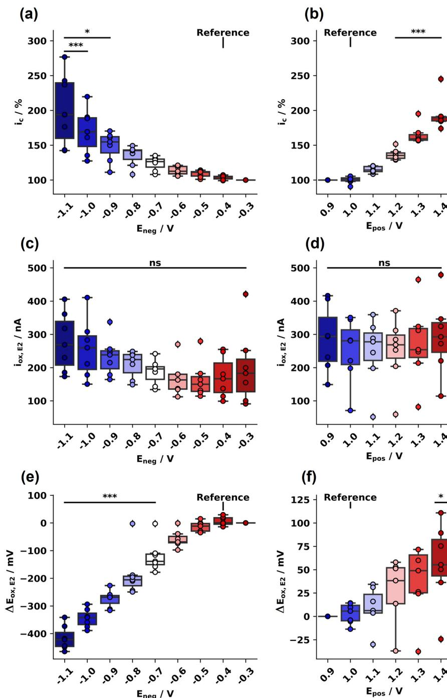
**Figure 3.** Variations of the capacitive current  $i_c$  with (a)  $E_{neg}$  and (b)  $E_{pos}$ . Variations of the anodic current  $i_{ox,E2}$  for (c)  $E_{neg}$  and (d)  $E_{pos}$  variations. Anodic peak potential shifts  $\Delta E_{ox,E2}$  for (e)  $E_{neg}$  and (f)  $E_{pos}$  variations. Post-hoc Tukey 95%, \*:  $p < 0.05$ , \*\*:  $p < 0.01$ , \*\*\*:  $p < 0.001$  vs. the reference dataset indicated in the figures.  $n = 7$ .
