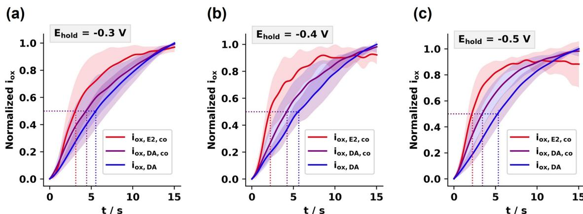
**Figure 12.** Dynamic response of the DA oxidative peak current for several  $E_{hold}$ .  $i_{ox,DA}$  is plotted over time from the injection point to 15 s after injection. The mean  $\pm$  standard deviation of  $i_{ox,DA}$  vs.  $t$  curves (3 to 5 measurements,  $n = 3$ ) are plotted for (a)  $E_{hold} = -0.3$  V, (b)  $E_{hold} = -0.4$  V, and (c)  $E_{hold} = -0.5$  V. The currents are normalised over their maximum values.
