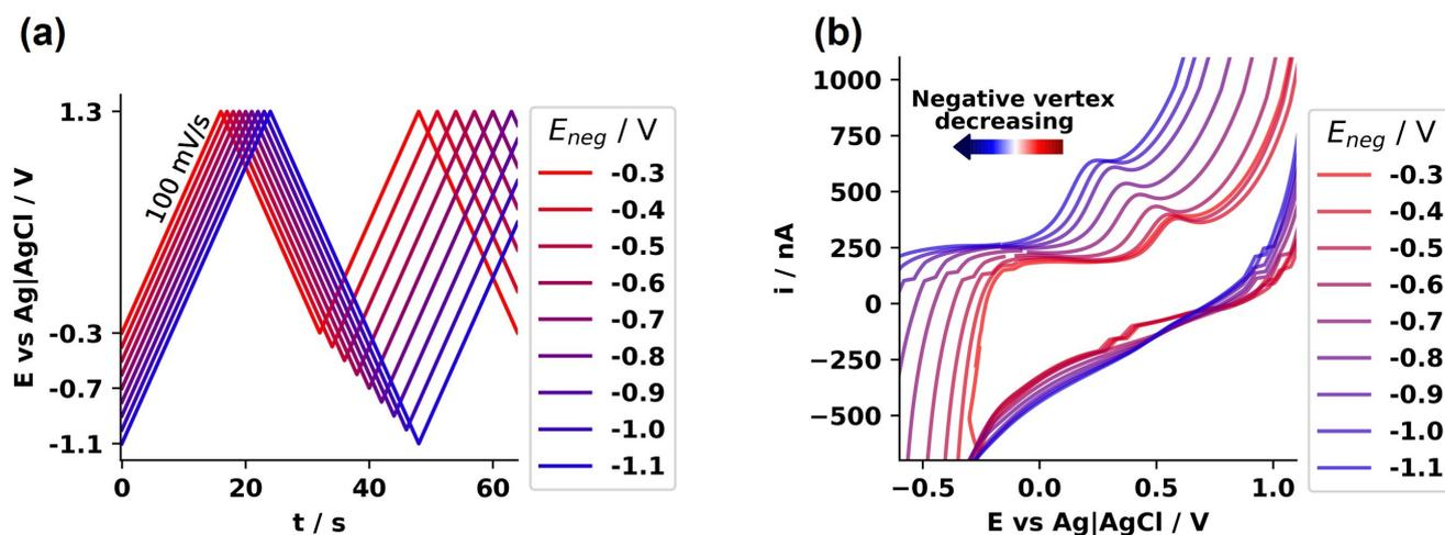
**Figure 1.** Negative vertex  $E_{neg}$  influence on E2 electrochemical response in CV. (a) Potential waveform applied for different  $E_{neg}$  ( $SR = 100 \text{ mV} \cdot \text{s}^{-1}$ ,  $E_{pos} = 1.3 \text{ V}$ ) and (b) the corresponding CVs.
