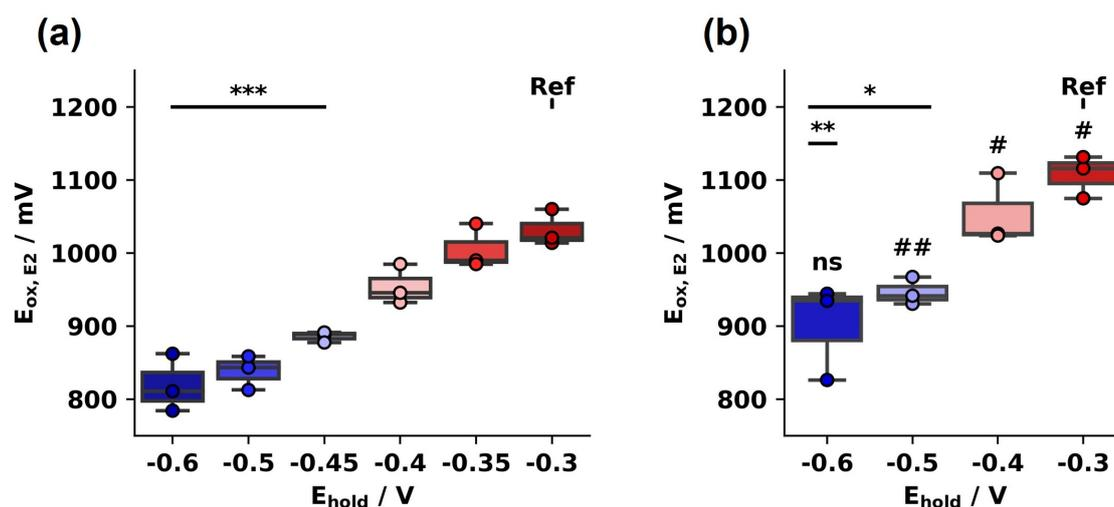
**Figure 7.** Impact of the holding potential  $E_{hold}$  on the position of the E2 anodic peak  $E_{ox,E2}$  for a positive switching potential  $E_{switch}$  of (a) 1.45 V and (b) 1.35 V. FSCV recorded for 10  $\mu$ M of E2 in PBS with 1% ethanol. Post-hoc Tukey 95%, \*:  $p < 0.05$ , \*\*:  $p < 0.01$ , \*\*\*:  $p < 0.001$  vs. the  $-0.3$  V dataset, and #:  $p < 0.05$ , ##:  $p < 0.01$  when comparing datasets for the same  $E_{hold}$  but different  $E_{switch}$ .  $n = 3$ .
