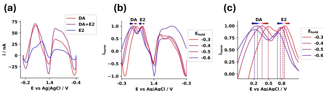
**Figure 8.** Codetection of E2 and DA using FSCV. (a) E2 peak is barely discernable when codetected with 1  $\mu\text{M}$  DA (purple curve). (b) and (c)  $\sim 7$  s after the injection point, E2 is more visible as the DA oxidation current increases slower than the E2 one. Both peaks shift to lower potentials with decreasing  $E_{\text{hold}}$ .
