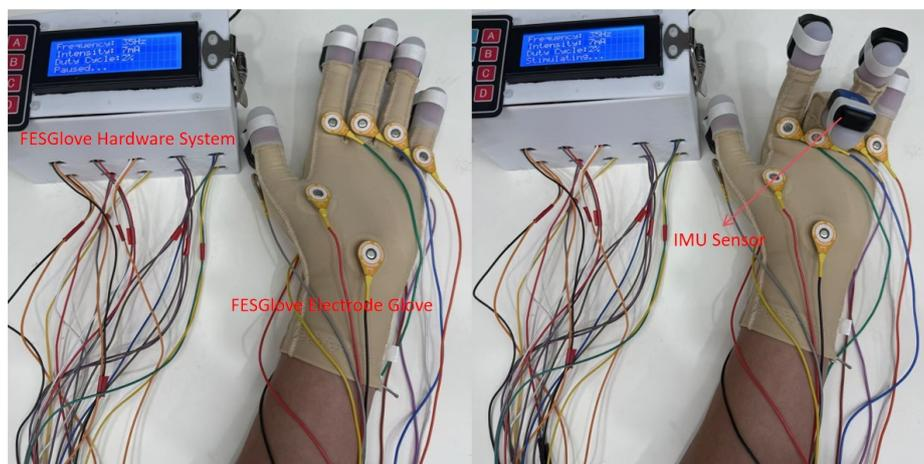
**Figure 9.** Experimental setup for independent single-finger control. It illustrates the experimental setup for evaluating middle finger flexion in one of the participants using the FESGlove system developed in this study.
