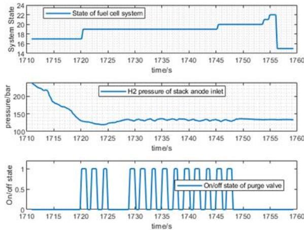
**Figure 13.** Parameter changes during shutdown process.
