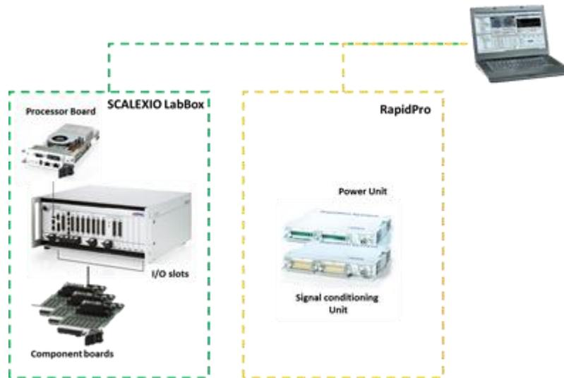
**Figure 2.** The composition of the hardware system of RCP.
