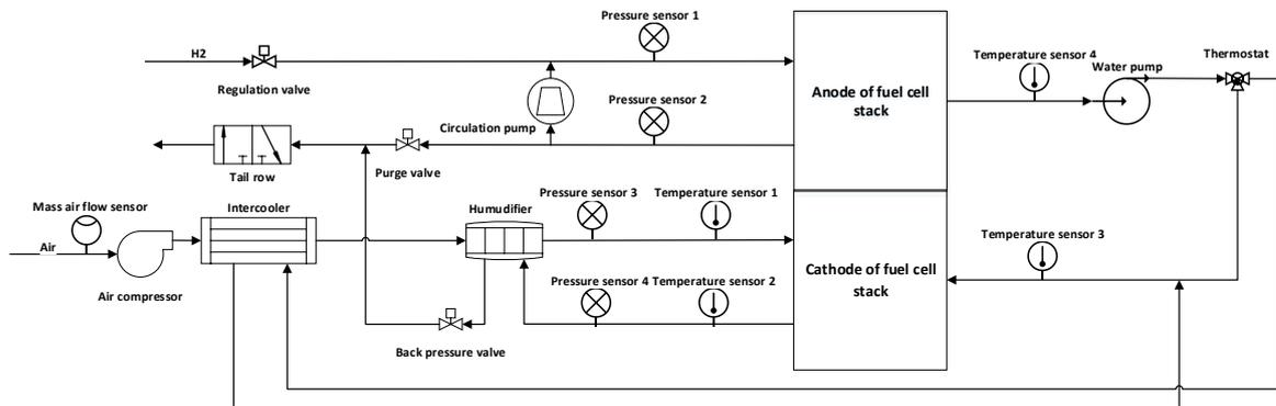
**Figure 6.** Fuel cell system architecture schematic.
